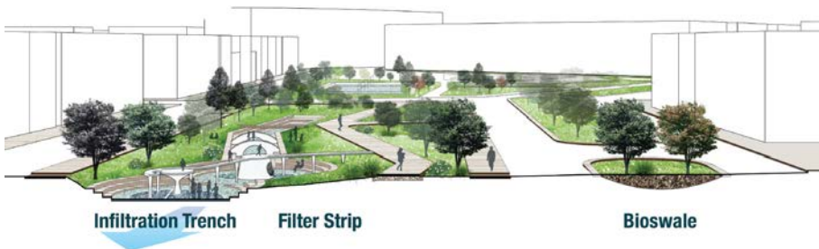
A green infrastructure proposal from one of the Georgia Tech studio teams. Not only does this proposal envision an infiltration area that helps slow down and clean stormwater, but it also provides a recreational amenity for families and residents that live near it.
