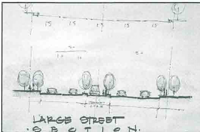
Typical Section of Large Street
